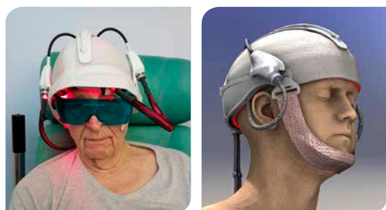
Picture of the Phosistos device for the photodynamic treatment of actinic keratoses of the scalp (on the left) and illustration of the modeling of 3D-printed helmet (on the right).
